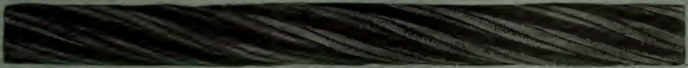
Illustration of 3/4" diam. Special Improved Patent Steel Wire Rope, 1760 yards long, supplied to Dalzell Colliery, Motherwell, Scot., which ran two years and 8 months, shewing condition when taken off. Previous rope from another maker lasted 1 year and 9 months
